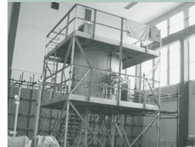
This Vinca critical assembly research apparatus once operated on weapons-grade HEU fuel. As a result of Project Vinca, it has been converted to proliferation-resistant low enriched uranium fuel.
