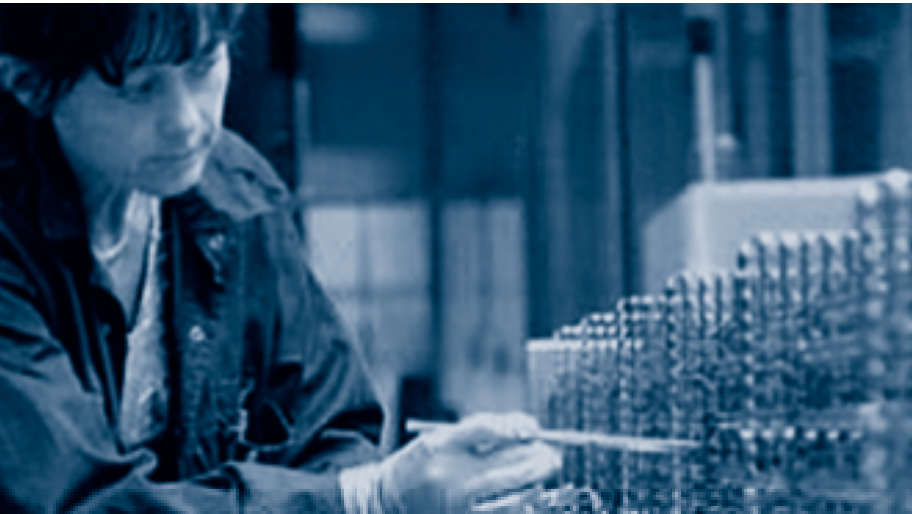
A technician checks nuclear fuel rods.
