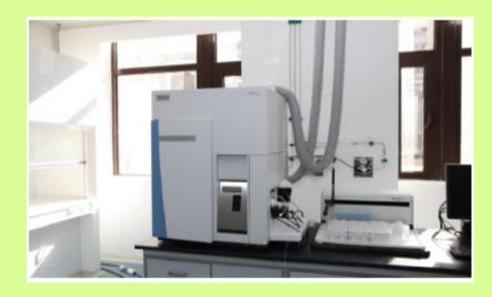
• TIMS, for measuring both isotope component and element content with high accuracy
