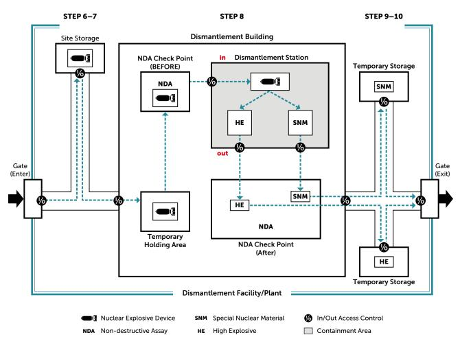
This chart was created to facilitate potential monitoring and inspection options at each step of the dismantlement process.
