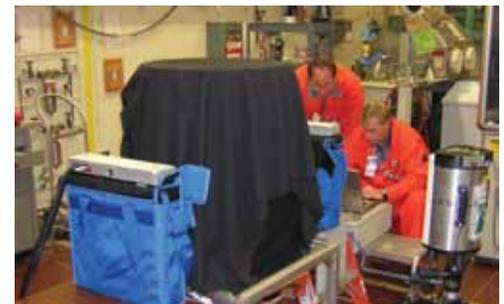
*Experts conducting neutron measurements on a concealed object during a U.S.-UK measurement campaign.*
