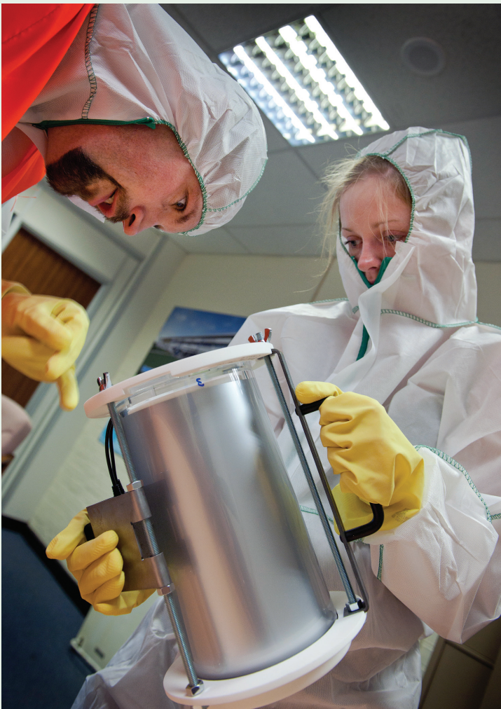
Monitor inspecting a video camera tamper-indicating enclosure during the Warhead Monitored Dismantlement Exercise.
