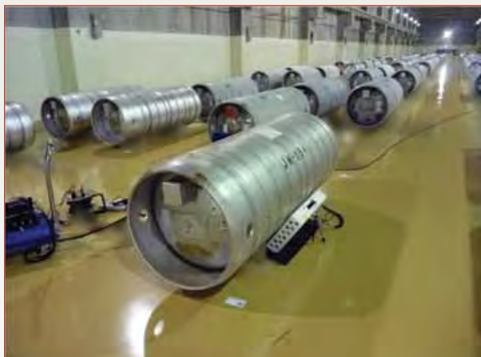
The Passive Neutron Enrichment Meter, being tested at the Rokkasho uranium enrichment plant in Japan.
