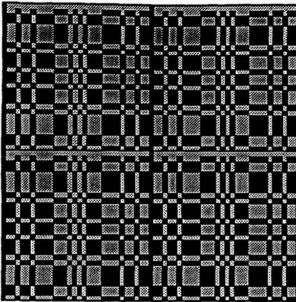
**FIGURE 1. UNIFORMLY REDUNDANT ARRAY OF APERTURES ARRANGED IN 4-FOLD MOSAIC OF 31 X 29 PATTERN**
