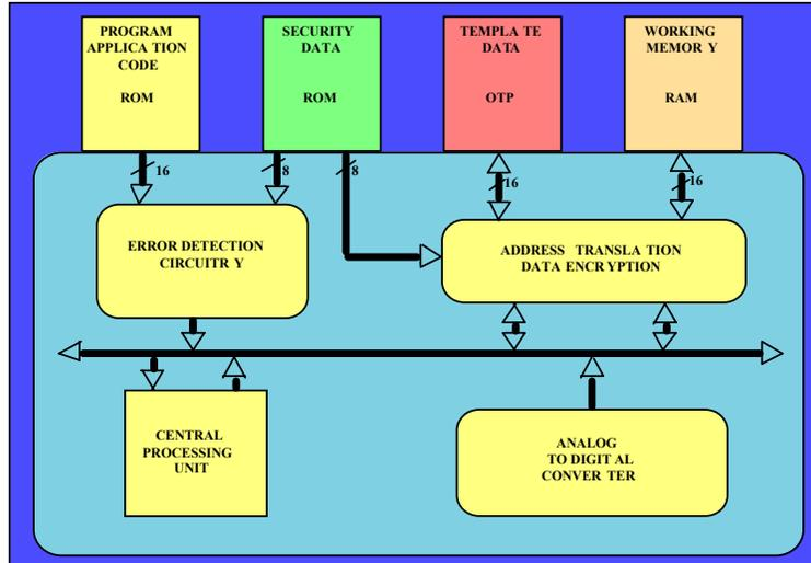
**Figure 2. Functional Schematic of CIVET Board**
