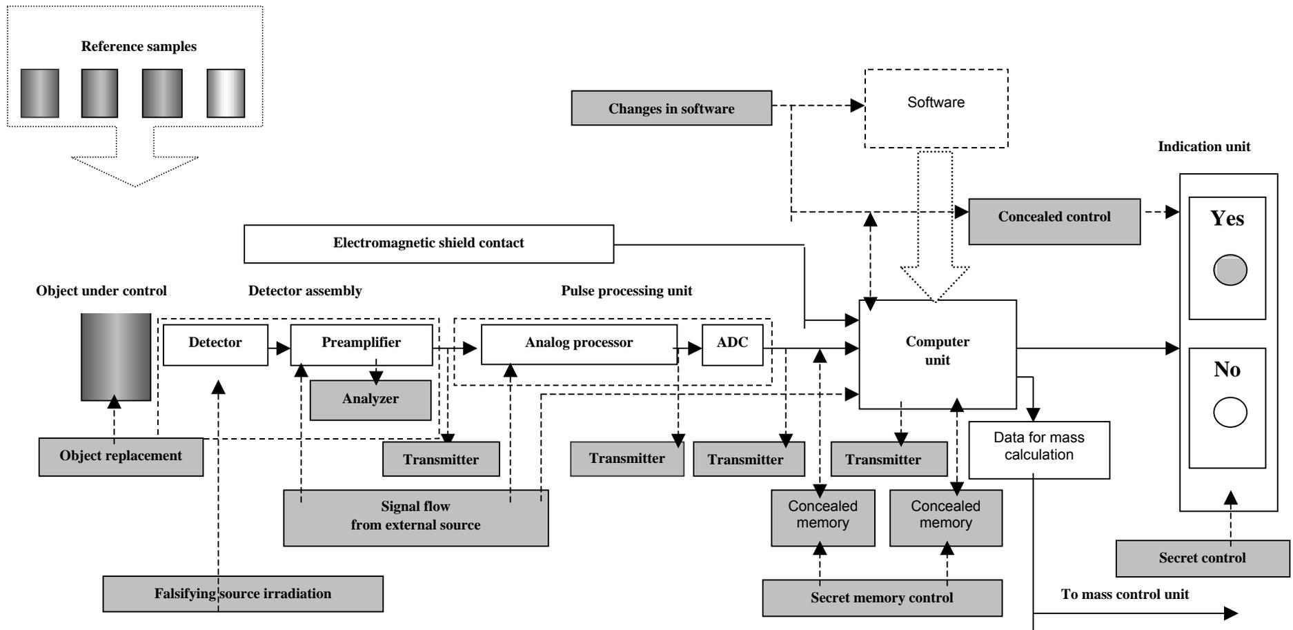
Fig. 3. The block diagram of a system for plutonium attribute control (determination of the presence of plutonium and the plutonium grade in the controlled object). Only one indication unit is shown. Grey colored blocks might be used for measurement intrusion (for explanations see text).
