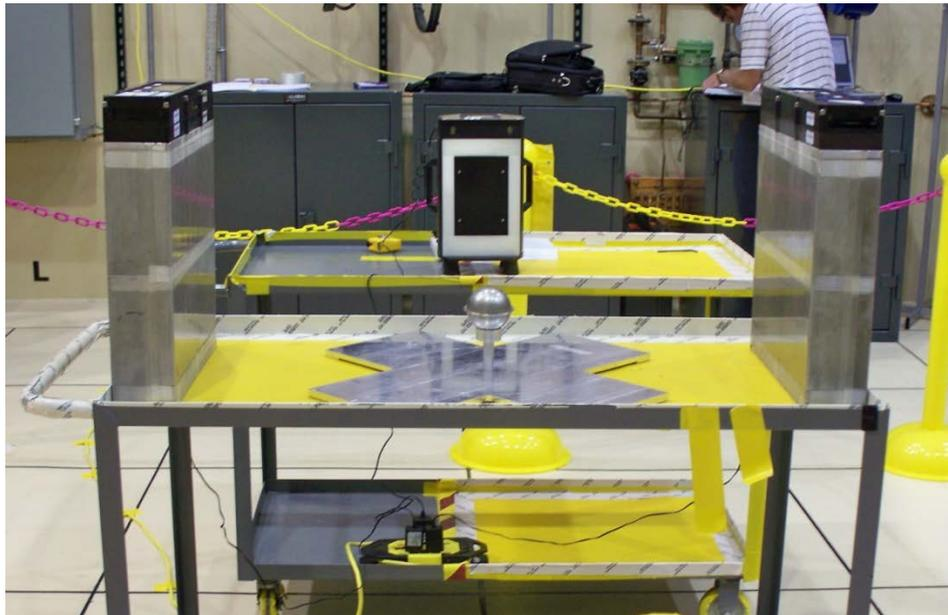
Figure 1: Default configuration: two NPOD3 detectors (left and right) and one SNAP detector (center, back) are used to measure the BeRP ball (center, front).
