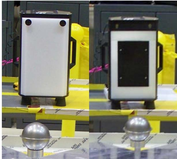
Figure 2: SNAP detector with polyethylene shield (left) and without.
