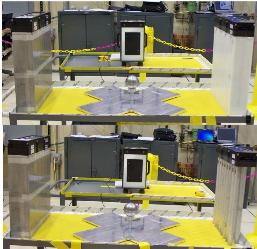
Figure 3: NPOD configurations - The NPOD on the left remained intact while the cadmium shield (top) and then the polyethylene moderator (bottom) were removed.
