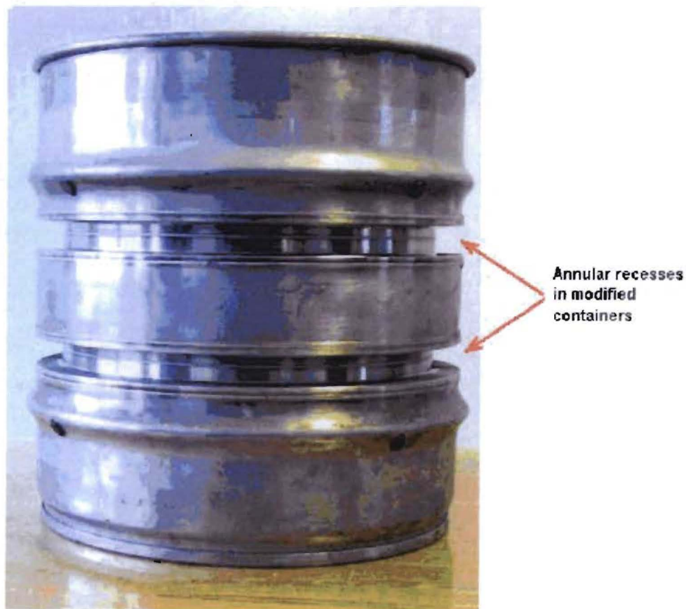
Fig. 2. Modified AT-400R container design highlighting changes to indicate unclassified contents.
