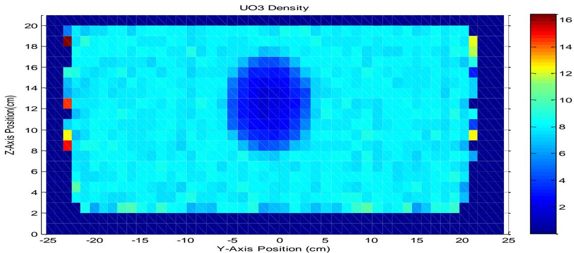
**Figure 6. A radiograph of unknown case number three showing the computed density of each pixel**
