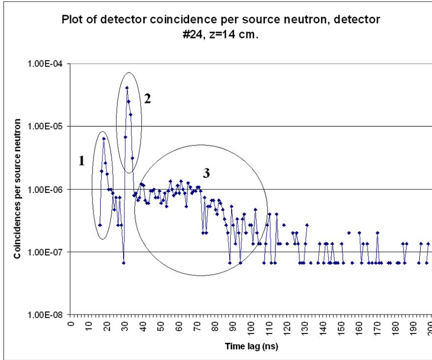
**Figure 3. Time-correlation graph of time-dependent source-detector coincidences with three regions of interest labeled.**
