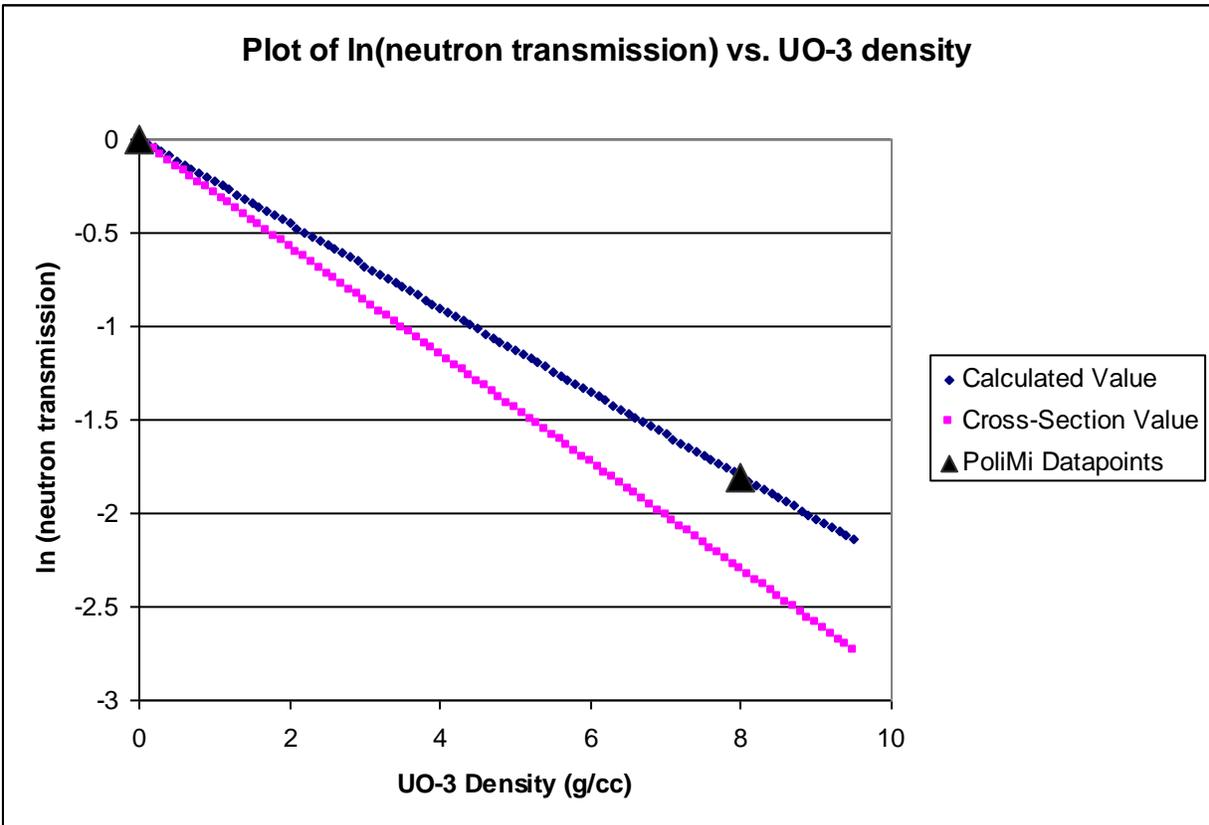
**Figure 4. A plot of the natural log of neutron transmission vs.  $\text{UO}_3$  powder density.**
