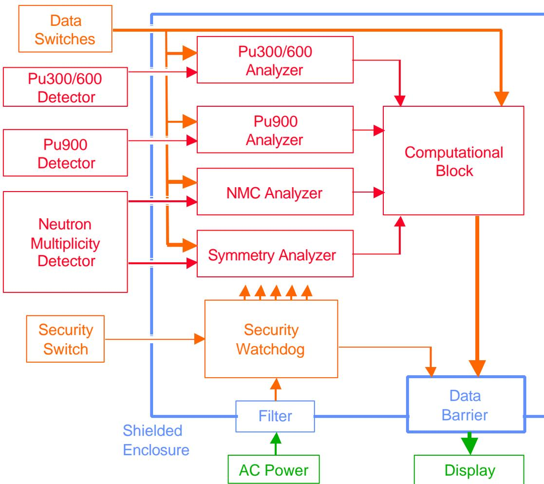
Fig. 1. Block diagram of attribute measurement system (AMS) for Mayak/PPIA. Elements that may contain classified information are shown in red. Elements that are themselves unclassified but must be treated as classified because of their location or function are shown in orange. Unclassified elements are shown in green. The protective enclosure and associated elements are in blue.
