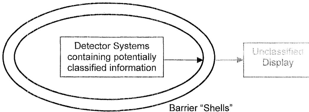
Conceptually, an information barrier can be viewed as series of nesting shells separating the classified information from the surrounding area. If all classified information is contained within this barrier, the level of protection depends more on the shells themselves and less on the details of the measurement systems within.
