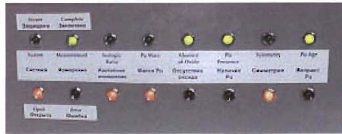
Fig. 4. Typical attribute display panel. Even displaying multiple attributes may not generate the same level of confidence as traditional data displays (e.g., neutron count rate or gamma spectra).
