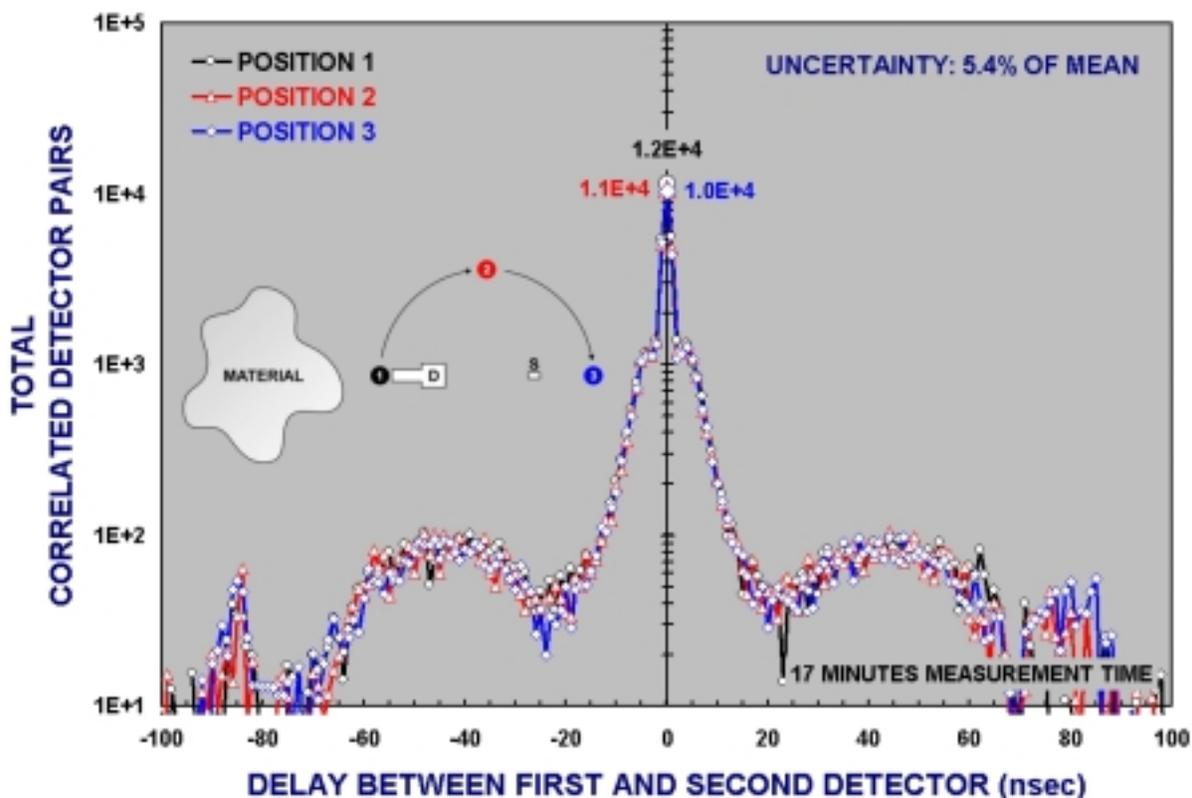
**Figure 2. Distribution of mutually correlated detection events measured for each orientation of the source and detectors relative to the external mass of fissile material. The source of the observed variability is self-correlated background emanating from the external fissile material.**
