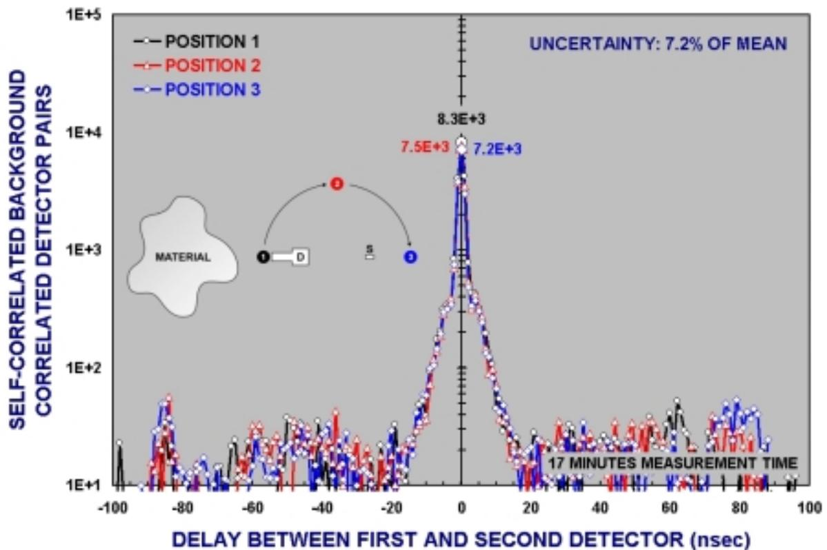
Figure 4. Distribution of mutually correlated detection events arising from self-correlated background measured for each orientation of the source and detectors relative to the external mass of fissile material. The source of the observed variability is the self-correlated background emanating from the external fissile material.
