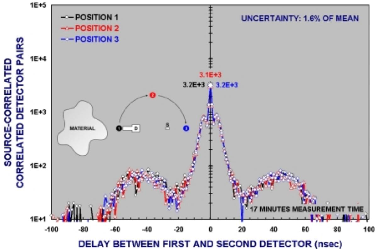
Figure 5. Distribution of mutually correlated detection events arising solely from the active source measured for each orientation of the source and detectors relative to the external mass of fissile material. This distribution is independent of all background, including self-correlated background. Consequently it does not vary significantly with proximity to external fissile material.
