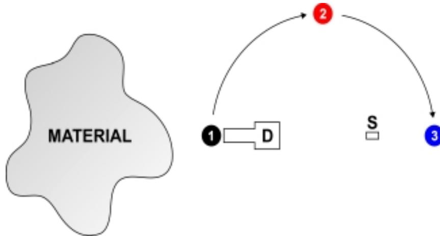
**Figure 1. Three test measurements performed using a  $^{252}\text{Cf}$  ionization chamber as the active source and an array of fast plastic scintillators to detect neutrons and gammas. The distance between the source (S) and the detectors (D) (approximately 1 m) was maintained constant while the orientation of the source and detectors relative to a mass of external fissile material was changed.**
