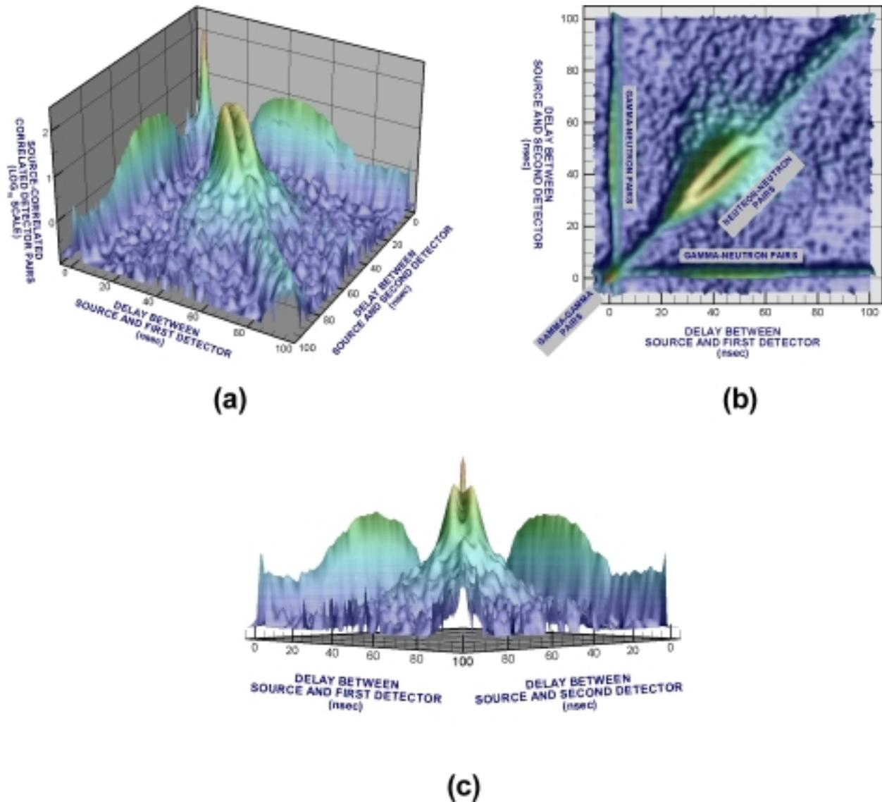
**Figure 3.** Distribution of mutually correlated detector count pairs that are in turn correlated to a source emission (a). Three classes of correlated detector pairs contribute to the distribution (b). The diagonal projection of the distribution illustrates the shape of the distribution of mutually correlated detector pairs arising solely from source emissions (c).
