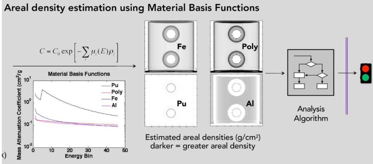
**Figure 2:** Overview of areal density estimation from material basis functions and a simulated AT-400R container. By using a Bremsstrahlung source and a photon-counting detector, materials in a radiograph may be distinguished. More details are given in [10].
