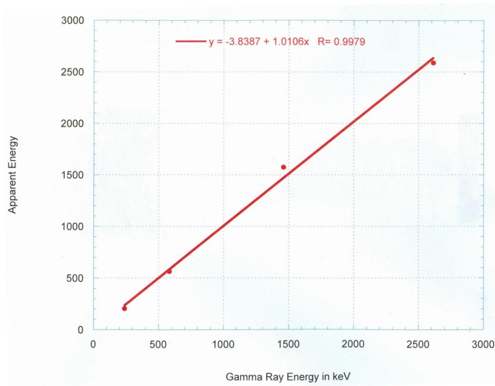
**Figure 4. Linear response of NG-TRIS using custom PMT base component.**
