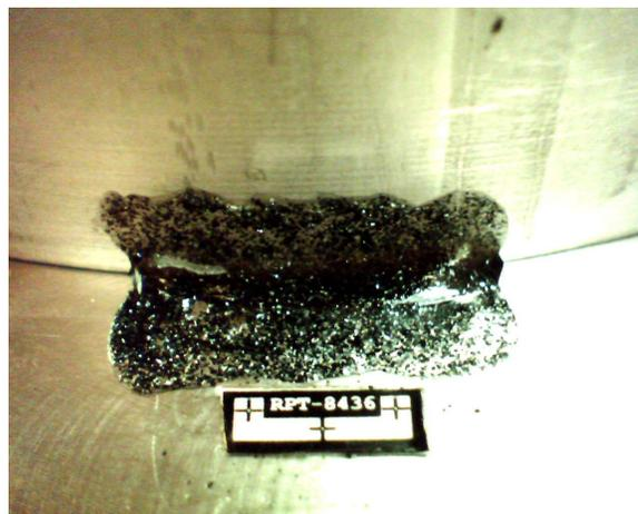
**Figure 2. Prototype RPT applied at the juncture of the NG-TRIS end plate and cylindrical case joint.**
