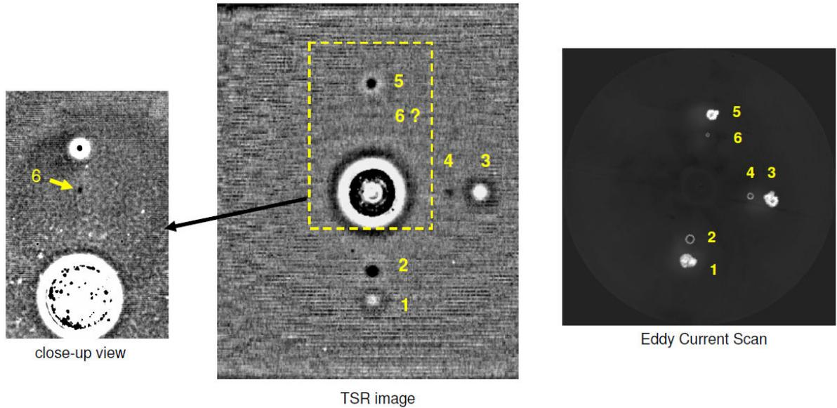
**Figure 1. Expertly drilled and repaired holes in the end plate of a steel case. The electrical connection is at center in each image above. Right: eddy current scan detecting 1/16", 1/8", 3/16" holes numbered 1 through 6. Center, and Left: pulse TSR image of the same holes.**
