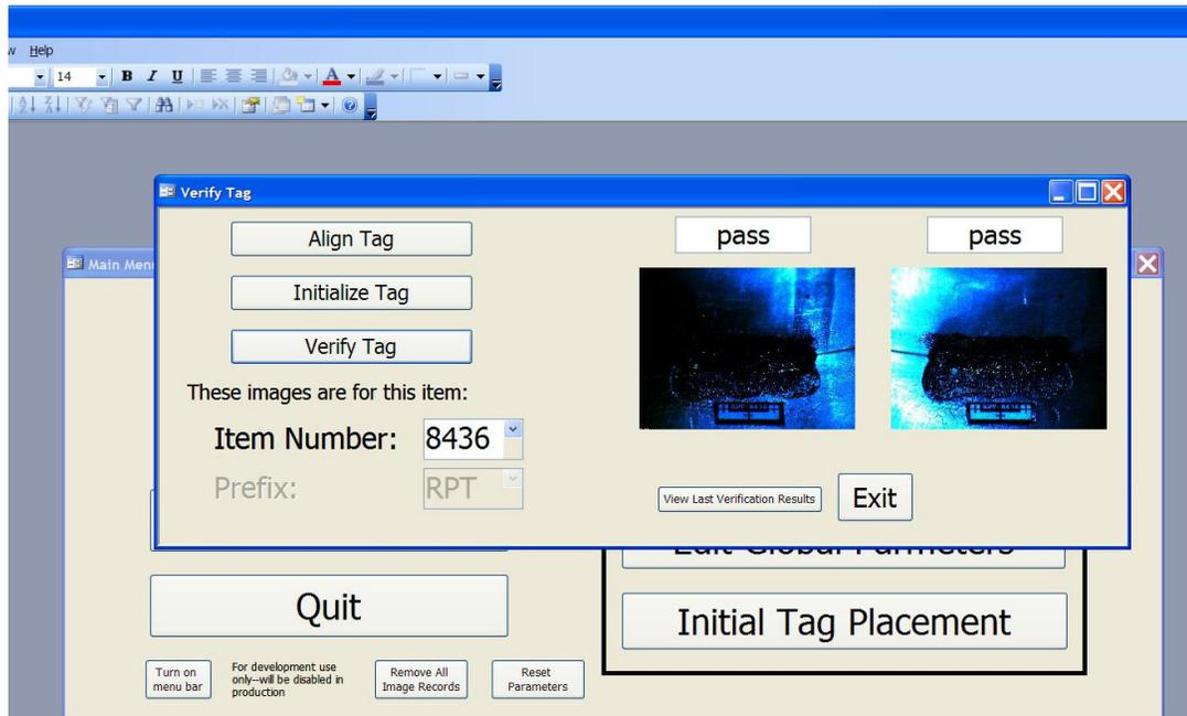
**Figure 3. Screen capture of the RPT reader showing a “Pass” condition for left and right illuminations of the NG-TRIS case joint tag.**
