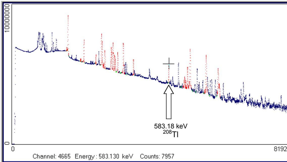
Fig. 6. Gamma ray spectrum from sample 26 with  $^{228}\text{Th}/\text{Pu}$  ratio =  $2.3 \text{ e-}010$ , the highest ratio found in this analysis. The 583 keV  $^{208}\text{Tl}$  peak is marked with the cross hair and arrow. Its intensity is not significant compared with the multitude of plutonium gamma rays. This sample is of European origin and is of a burnup far in excess of weapons grade specifications.
