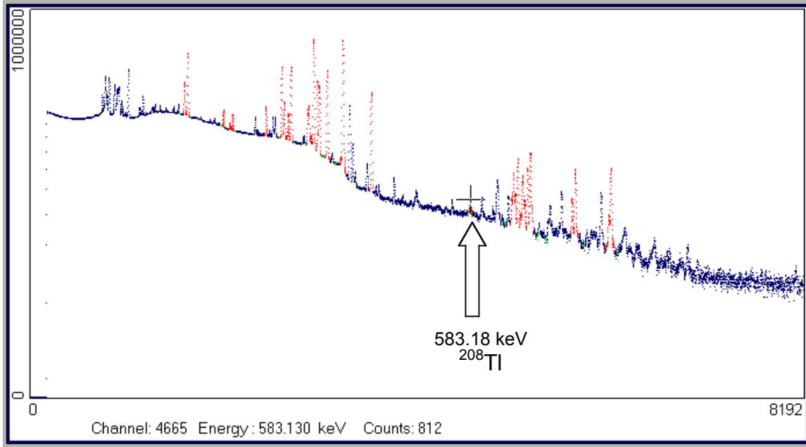
*Fig. 5. Gamma-ray spectrum from sample 6 with  $^{228}\text{Th}/\text{Pu} = 2.2 \text{ e-}012$ , a typical number for weapons-grade plutonium found in this analysis. The 583 keV  $^{208}\text{Tl}$  peak is marked with the cross hair and arrow. The intensity of this peak is insignificant.*
