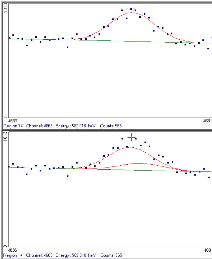
Fig. 1. These two figures show the 583 keV region from sample 4, a weapons-grade plutonium sample with 6% Pu-240 and a very small Tl-208 content. The top picture shows the envelope of the fit of the two peaks. The individual components are shown in the bottom picture. The smaller component is the 583.187 keV gamma ray from Tl-208, while the larger component is the 582.89 keV peak from Pu-239. The energy of the channel denoted by the cross hair is shown at the bottom of each frame.
