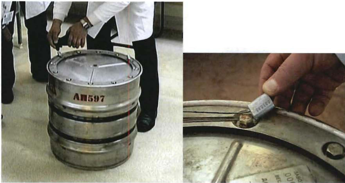
Figure 3 Left: seal being applied to the AT400R containing the one of the RM after the acceptance tests at IPPE. Right: Seal being checked during the demonstration at VNIIEF.
