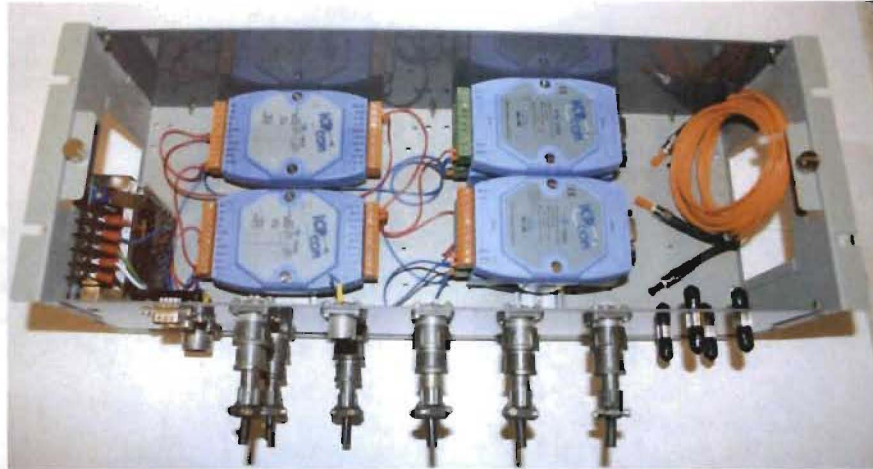
Figure 2 The custom electronics were made using easy-to-understand I-7000 series modules.
