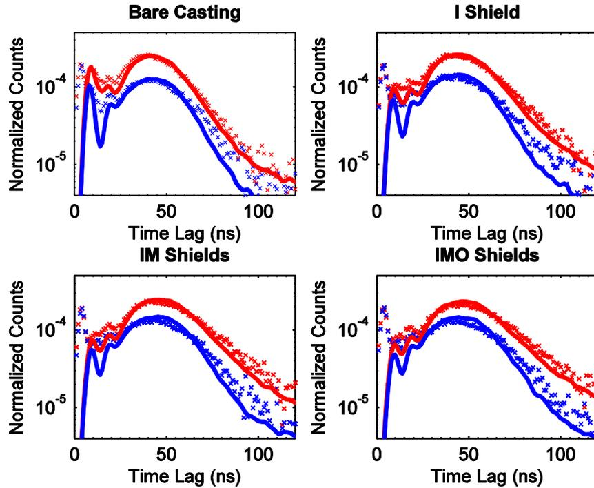
**Figure 7. Comparison of simulations and measurements for all the shield combinations using detector #5 and pixel #11 of the  $\alpha$  detector. The solid lines are simulations, and the x's are measurements.**
