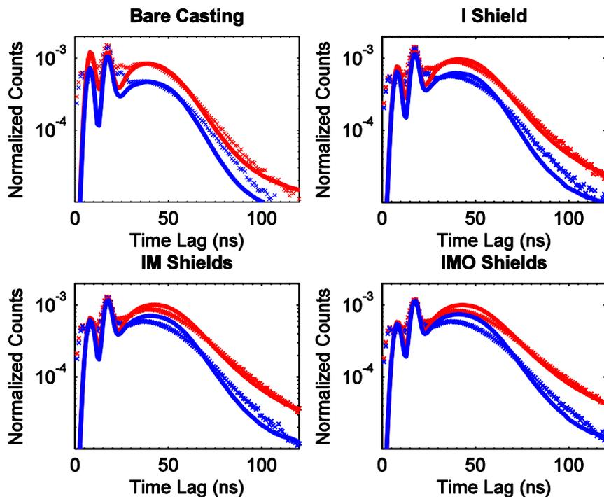
Figure 6. Comparison of simulations and measurements for all the shield combinations using the top row detectors and all pixels of the  $\alpha$  detector. The solid lines are simulations, and the x's are measurements.
