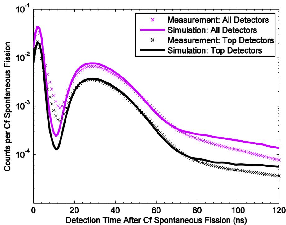
Figure 4. Comparison of the  $^{252}\text{Cf}$  measurements and simulations.
