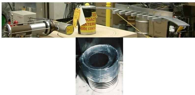
**Fig. 3. Source-uranium metal-casting-detector configuration for imaging.**
