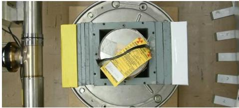
**Fig. 6. DU casting with 1-in.-thick lead box surrounding and 4-in. thickness of lead plates in front and back.**
