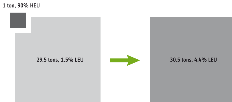
Figure 2.1. Schematic showing amount of 1.5-percent enriched blend-stock required to blend down one ton of excess 90-percent enriched Russian
