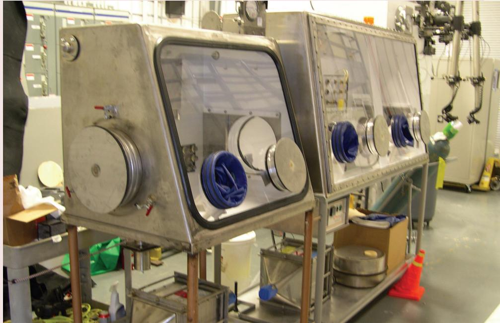
Glove boxes being prepared for the processing and qualification of the recovered U-233 items.
