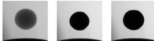
Figure 7: Example active images of spherical objects. Images of a rubber ball (left), quartz ball (middle), and marble (right).
