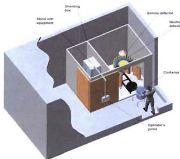
Fig. 4. Conceptual drawing of the AVNG. This system measures neutrons and gamma rays and incorporates the AMS and IB features outlined in this presentation.
