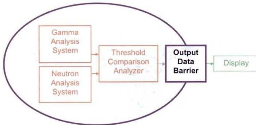
Fig. 2. An example of an AMS incorporating neutron and gamma detection systems. The Russian AVNG and similar systems use  $^3\text{He}$ -based neutron detectors and high-purity germanium (HPGe) gamma detectors. Components potentially containing classified information are shown in red, IB components in purple, and unclassified components in green.
