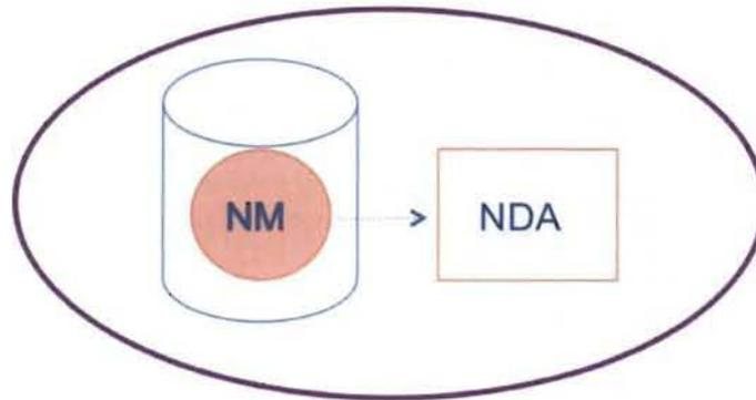
Fig. 1. A conceptual IB. The nuclear material and all measurement equipment are surrounded by a barrier that keeps any classified information inside and monitoring party outside.
