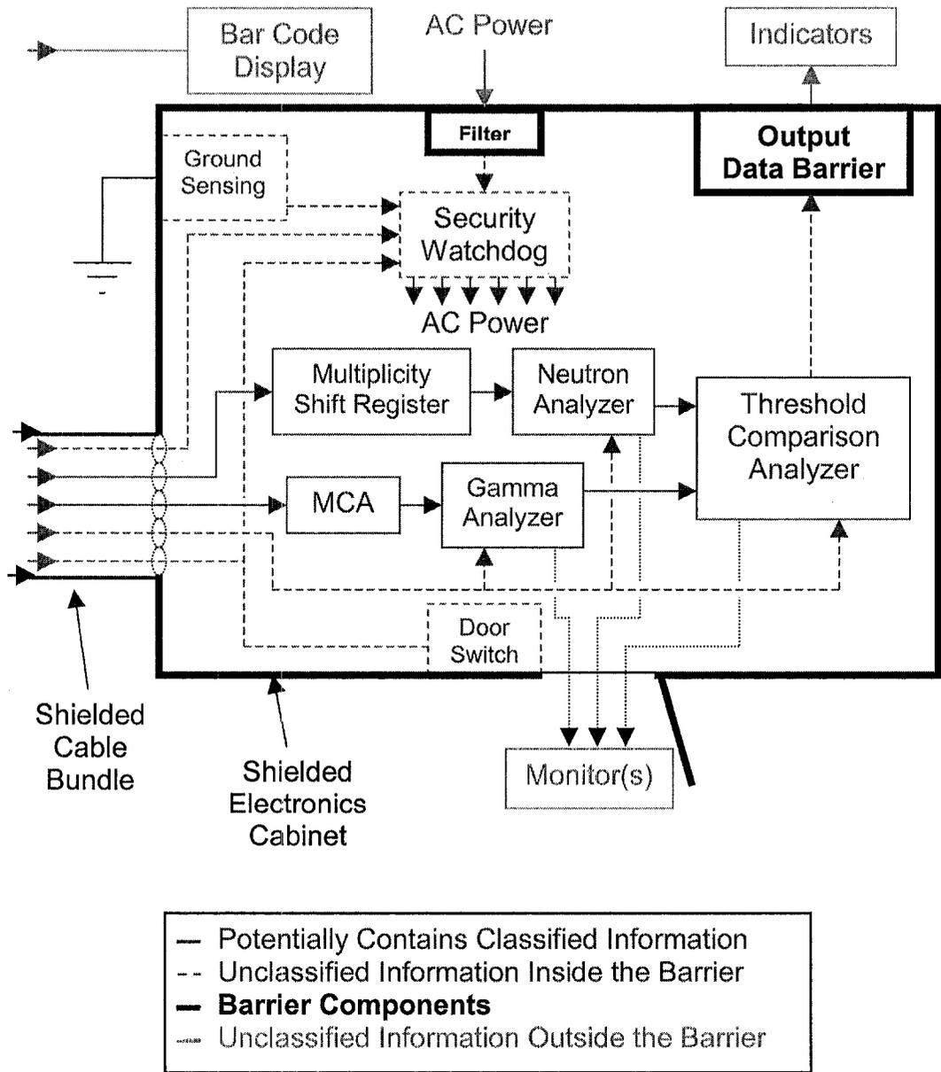
Fig. 2b. The second half of the AVNG. This illustration contains all of the data analysis components as well as the unclassified indicator display. The monitors that can be connected to the AVNG during unclassified measurements are also illustrated. The AVNG is illustrated in the open mode. If the video monitors were removed and all access doors closed and interlocked, then the AVNG would be in the secure mode.
