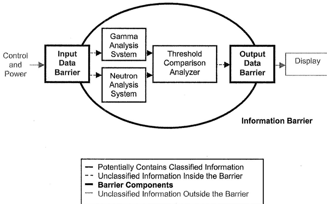
*Fig. 1. Core concept of an attribute measurement system. The data barriers are the only points of contact between the internal computing systems and the unclassified display and controls.*
