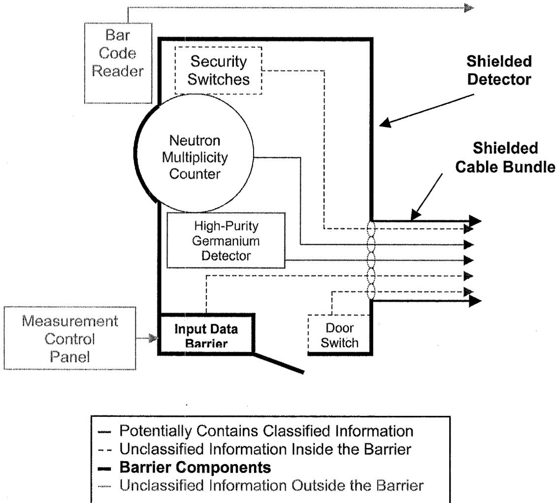
*Fig. 2a. Detectors and detector enclosure for AVNG. This figure also includes all operator switches (the measurement control panel) as well as a bar code reader to register the identity of measured containers.*
