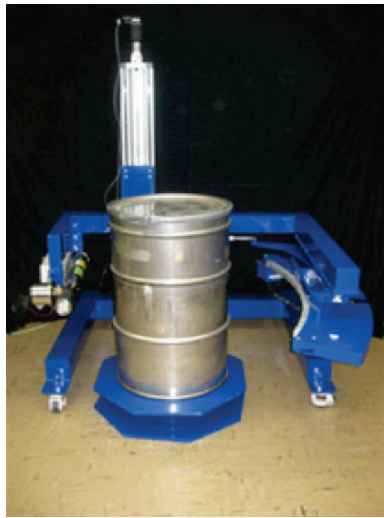
Figure 2. NMIS scans in ways similar to tomographic scanners. The turntable (c the scanned container (e.g., a drum); th vertically positions the neutron generat
