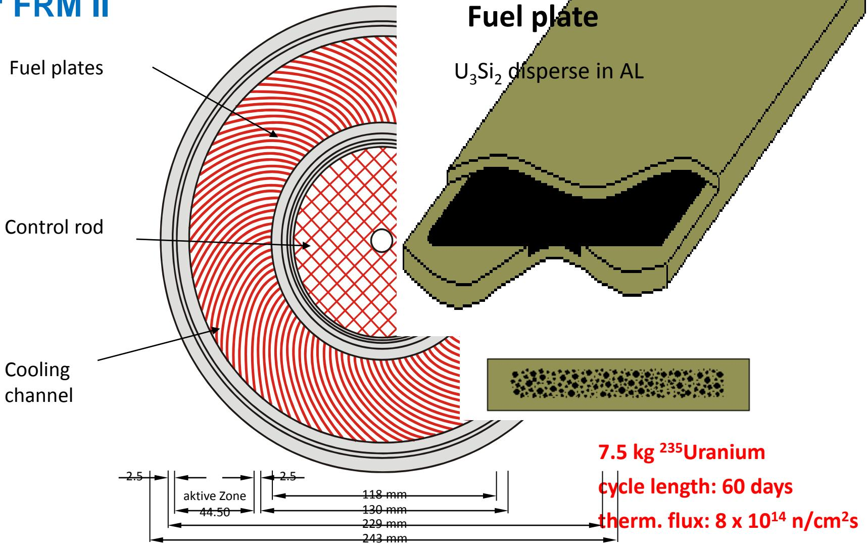
$\text{U}_3\text{Si}_2$  is an approved and reliable alloy for high performance research reactors.
