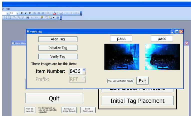
**Figure 10.** Inspector interface showing right and left illuminations for RPT validation.
