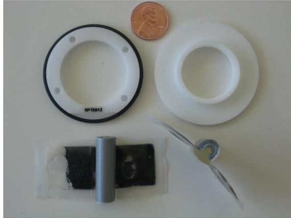
**Figure 3.** The mechanical alignment tag frame (left, top), with bubble packs (bottom) for dispensing a two component epoxy and particle mixture, and tag stencil (top, right).
