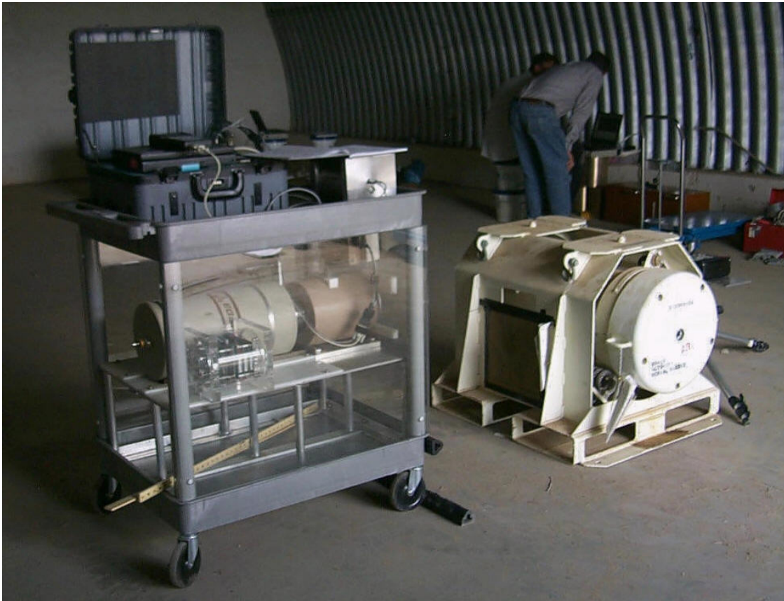
Fig. 1. The TRADS uses a HPGc detector to confirm attributes of the inspected item, which is a W84 warhead in this photograph. The trusted processor and electronic components are placed on top of the cart in which the detector is mounted. The trusted processor is the silver object at the upper-right corner of the cart.
