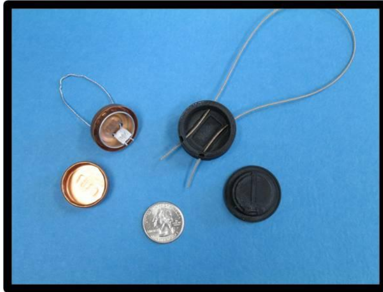
Figure 1: Size comparison of a metal seal (left), rapid-prototype mockup of the ITICS (right), and a U.S. quarter (bottom). Picture courtesy SNL.
