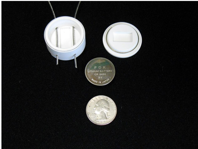
Figure 3: First prototype seal base with wire (left), seal cap with snap ring (right), battery (center), U.S. quarter (bottom) for size comparison. Picture courtesy SNL.
