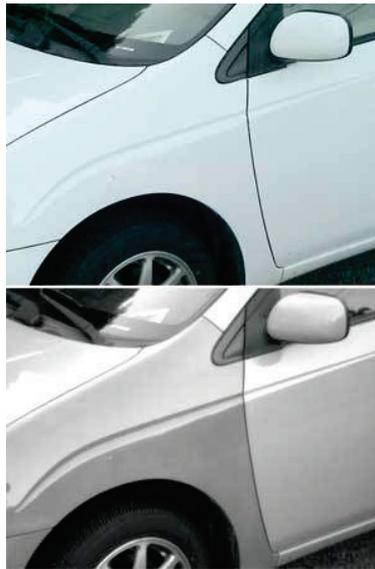
**Figure 5:** The top picture shows a vehicle whose front fender has been replaced imaged in the visible band, and the bottom picture shows the same vehicle imaged in the 320 – 400 nm UV band [8].
