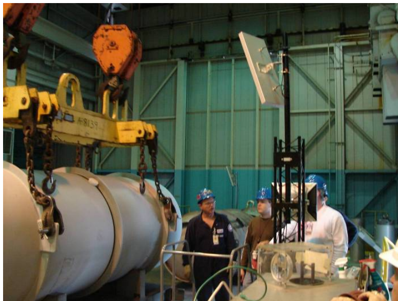
Figure 5: RF monitoring as cylinder is moved to scale for post process weighing.
